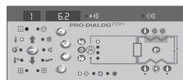
Pulpit operatora sterowania Pro-Dialog Plus
